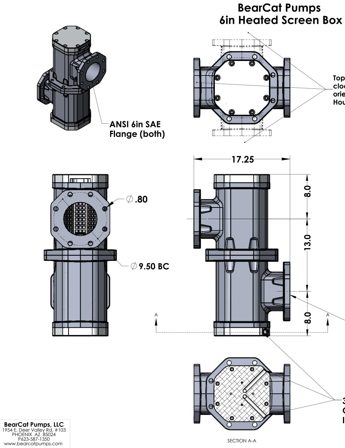
Top Plate V75-369 oring Top Housing can be clocked in any 90deg Basket oriention to bottom Housing Top Housing Heat Column Bottom Housing (2) V75-373 oring Mid Section and Base Plate Flange to pump V75-369 oring V75-234 oring -3/4 MJIC/MB Hot **Oil Connections** Inlet and Oulet REV Page 1 OF 1
