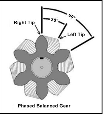
stabilized flow increases accuracy in the meter and at the same time raises the cavitation point (and maximum flow) of the pump.
