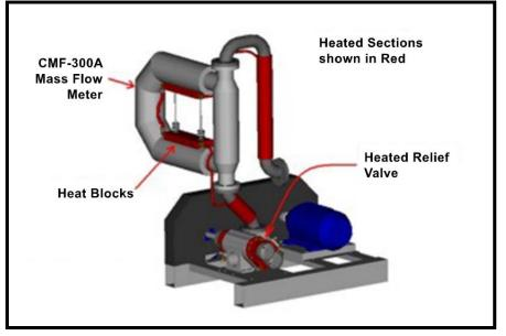
Coupled with a heated relief valve, the heat blocks complete a system that is able to purge and circulate rubberized asphalt. This works because it provides three valuable functions that were absent in previous systems; a meter that can withstand higher temperatures, oil traced heat blocks to safely heat the meter with the existing transfer oil, and a heated relief valve so that a safe level of pressure can be applied to slowly purge blockages from the system.
