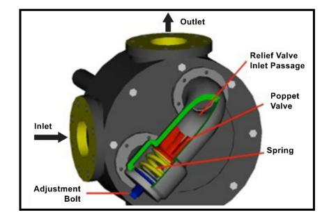
• The vast majority of the pumps used in the asphalt industry have a *non-heated relief valve*. We believe this to be a significant problem. Consider the following:
