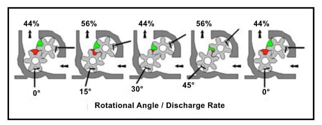
The above graph shows the rotation of  $60^{\circ}$ . The position of  $0^{\circ}$  and  $30^{\circ}$  are symmetrical in displacement at a rate of 44%. While 15° and 45° discharge at a rate of 56% of the total tooth volume. This correlates to 12 pulses per revolution.
