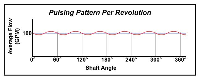
While much has been done within the electronics to filter the pulsing within the meter itself, there is still a potential for these pulsations to affect the operational frequencies of the coil and pick off sensors.
